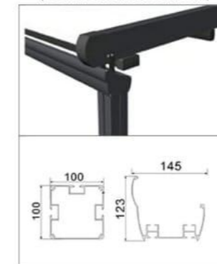
A: Column and water tank (Suitable for under 5 meters)
